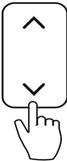
**ADJUST button:** Used to choose functions or adjust parameters. On parameter unadjustable interface, press the "▼" & "▲" button to select the specified function in a range of F1 ~ F9 and E1~E9. Then pressing the **MODIFY** button to enter the parameter modifying interface, the relevant parameter flashes, pressing "▼" & "▲" button to adjust the parameter.
