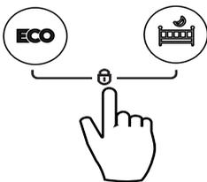
**LOCK button:** Hold and press these two buttons for 2 seconds, all current settings of indoor unit are locked in and the remote controller does not accept any operation except that of the LOCK.
