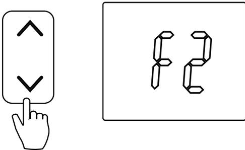
2. Press **MODIFY** button. Then press "**^**" & "**∇**" button to choose the parameter. The parameters can be adjusted within a range of  $-6^{\circ}\text{C}$ ~ $6^{\circ}\text{C}$ .
