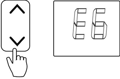
2. Press **MODIFY** button. Then press "▲" & "▼" button to choose the network address between 0 to 63 or "--".
