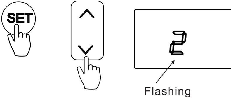
3. Press **MODIFY** button to adjust the parameter in the range of 8°C~28°C.
