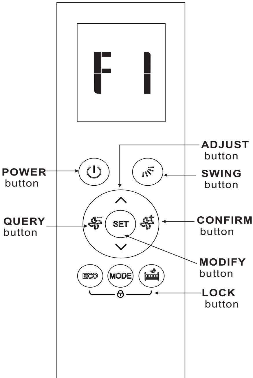
**IMPORTANT:** The remote controller is only enabled within 10 minutes after the indoor unit is powered on, and the indoor unit must be switched off.
