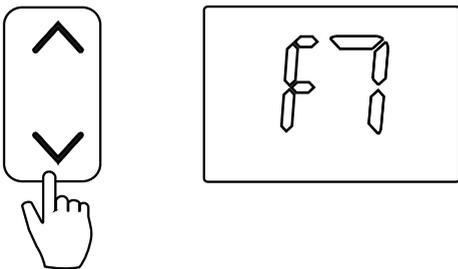
2. Press **MODIFY** button. Then press " ^ " & " v " button to choose the parameter in a range of -2°C~2°C.
