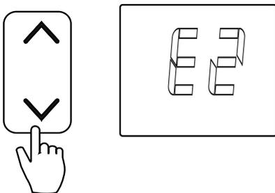
2. Press **MODIFY** button. Then press "▲" & "▼" button to set the temperature in a range of 17°C to 24°C.
