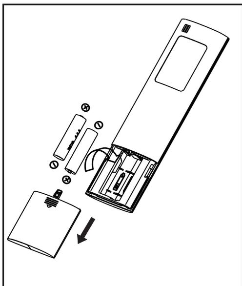
The remote controller uses two alkaline dry batteries (R03/LR03X2)
