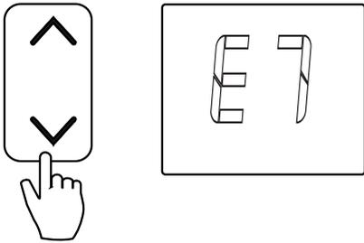
2. Press **MODIFY** button. Then press "▲" & "▼" button to choose the capacity code between 0~11.
