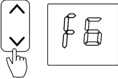
2. Press **MODIFY** button. Then press " ^ " & " v " button to select "HH" or "CH". (HH: Heating only, CH: Cooling & Heating)
