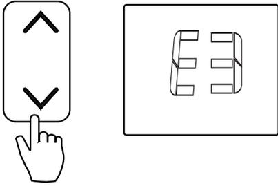
2. Press **MODIFY** button. Then press " ^ " & " v " button to set the temperature in a range of 25°C to 30°C.
